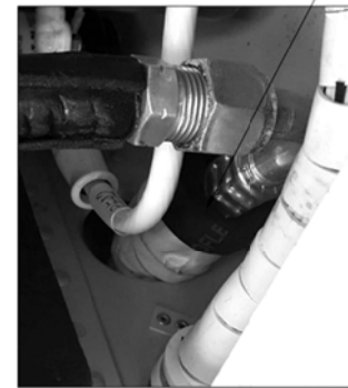
DETAIL '2' - REFRIGERANT LINE LOCATED UNDER EVAPORATOR
